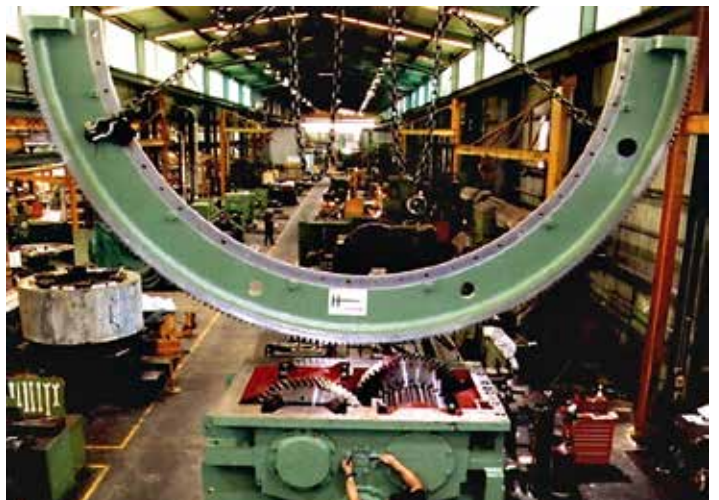
SELF ALIGNING, TWIN PINION MILL DRIVE GEARBOX
