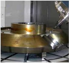
An extensive collection of 5-axis machines to cut spiral, helical and straight bevel gears and worm wheels. Unique software is used to optimise the CAM program for the manufacture of spiral, helical and straight bevel gears and worm wheels.
