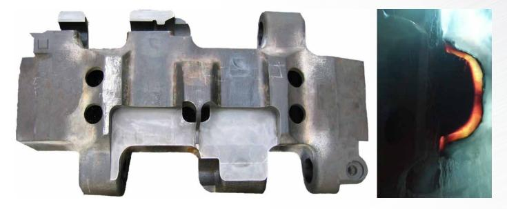
Drive lugs, roller surfaces and pin bores can be induction hardened. Alternatively, bores can be fitted with case hardened bushes (carburised to 3mm). Pins are normally made of either 4140 or 4340 and are quenched, tempered and induction hardened to the required depth. Case carburised pins are available for extreme working conditions where the pins have proved to be wearing excessively.
