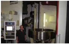
SLEW BEARINGS - Induction hardened and precision ground
