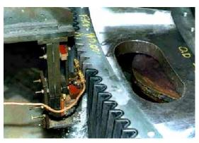
Computerised full contour induction hardening of large Slew gears and bearing race ways.
