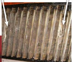
Forged steel fabricated girth gears overcome cast steel cracking problems. Forged steel gives the highest crack and impact resistance.
