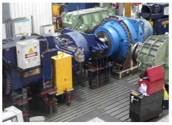
Above: Hofmann refurbished P2SA-38 (2800kW) HPGR Gearbox under load test.
