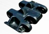
Induction hardened alloy steel. Induction hardened bores, roller path and drive lug.
