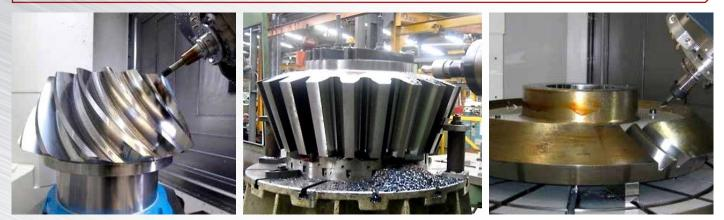
An extensive collection of 5-axis machines to cut spiral, helical and straight bevel gears and worm wheels. Unique software is used to optimise the CAM program for the manufacture of spiral, helical and straight bevel gears and worm wheels.
