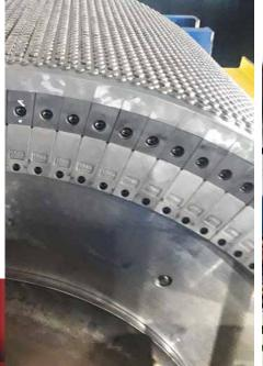
Tungsten carbide blocks, bolt on retaining clamp plates and soldered Tungsten Carbide pieces (Patent no: 2011301142). Individually clamped • Can't break off Individual blocks can be replaced.
