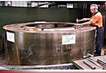
ROLLS CRUSHERS - HARD FACED, WHITE IRON & SEGMENTED
